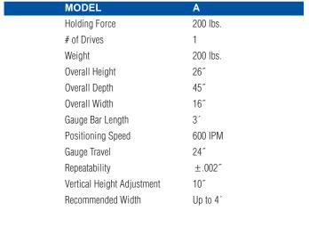
The A compact gauge for press brakes with 12" to 42" between sideframes. This unit is available with a 3' gauge bar for light applications.
