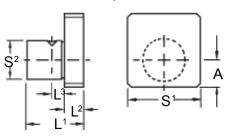
Adapter face will accommodate mounting & dowel holes for standard or special punch retainers.
