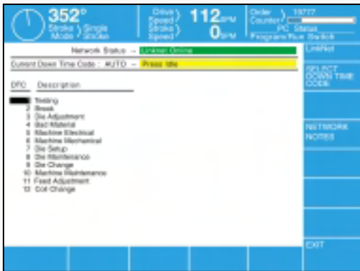
Down time codes as they appear on the OmniLink 5000 screen.
