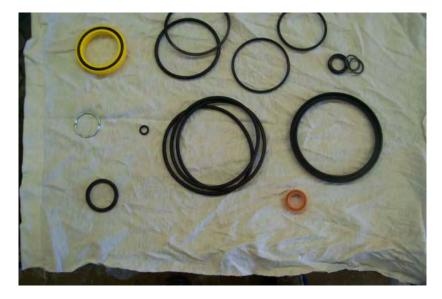
Lay out and grease all seals from seal kit. It is very important to grease the seals to avoid tearing during installation.
