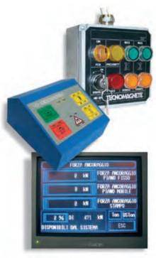
On request Quad Stamp is supplied with IPC interactive power control push-button. Through a touch-screen it is possible to control all the system functions and display the actual force generated by the magnet on each different die.
