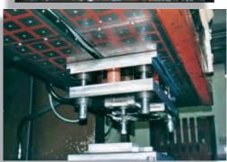
If the die is not magnetic or when the contact surface die/magnet is too small, the die can be equipped with a common steel backplate
