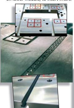
The UR ("U-Rail") version is made in separate parts, for free and flexible positioning on the machine platen to insert "U channel lifters" of different sizes.
