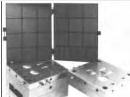
Interior actual FORTAL mold cavity specimen surface finishes have been creating permitting the user to make side-by-side finish comparisons. Built for shop floor use.
