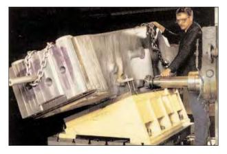
**FRAME MACHINING AND REPAIR** Used frames are sandblasted and inspected for cracks and wear. All frame areas – guide pockets, top and base surfaces – are machined as a matched pair. Superior has the patterns and capabilities to furnish new cast steel frames.
