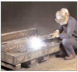
**WELDING** Superior's welding craftsmen use MIG, TIG, and submerged-arc welding in manufacturing and repairing forging hammer and press components.
