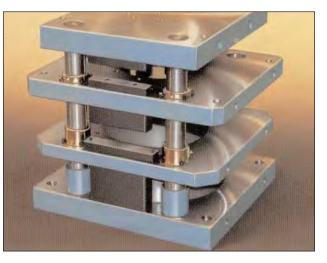
Complex, multi-platen trim die sets and tooling are engineered, manufactured, and assembled at Superior in coordination with customer forging engineers.
