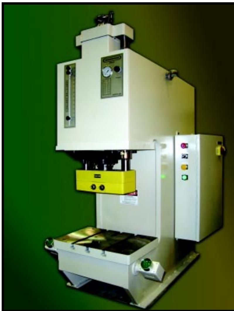
Pressure easily adjustable on up-front control panel.
